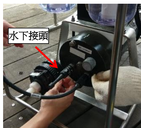
Figure 27: 將水下接頭移除並連接電腦
