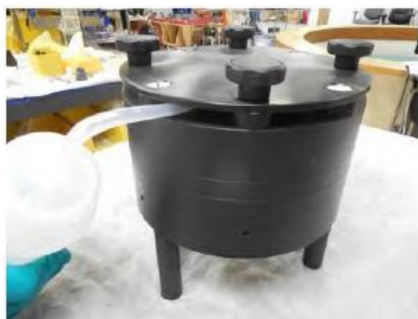
Figure 23: 將水注入頂層
