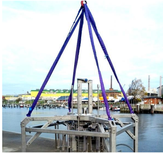
Figure 7: Multi Corer hooked on to the 4 lashing points
